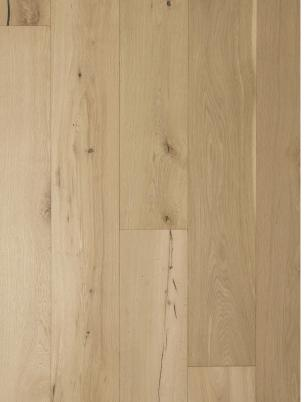
Campania's wear layer is constructed from 4mm solid European White Oak Hardwood and its core is comprised of layers of plywood. Straight Plank flooring is one of the most sought after hardwood choices in the US. All of these layers combined result in a 5/8" total plank thickness and each plank measuring 7-1/2" in width.
