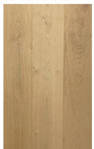
Unfinished (7.5)'s wear layer is constructed from 4mm solid European White Oak Hardwood and its core is comprised of layers of plywood. Straight Plank flooring is one of the most sought after hardwood choices in the US. All of these layers combined result in a 5/8" total plank thickness and each plank measuring 7-1/2" in width.
